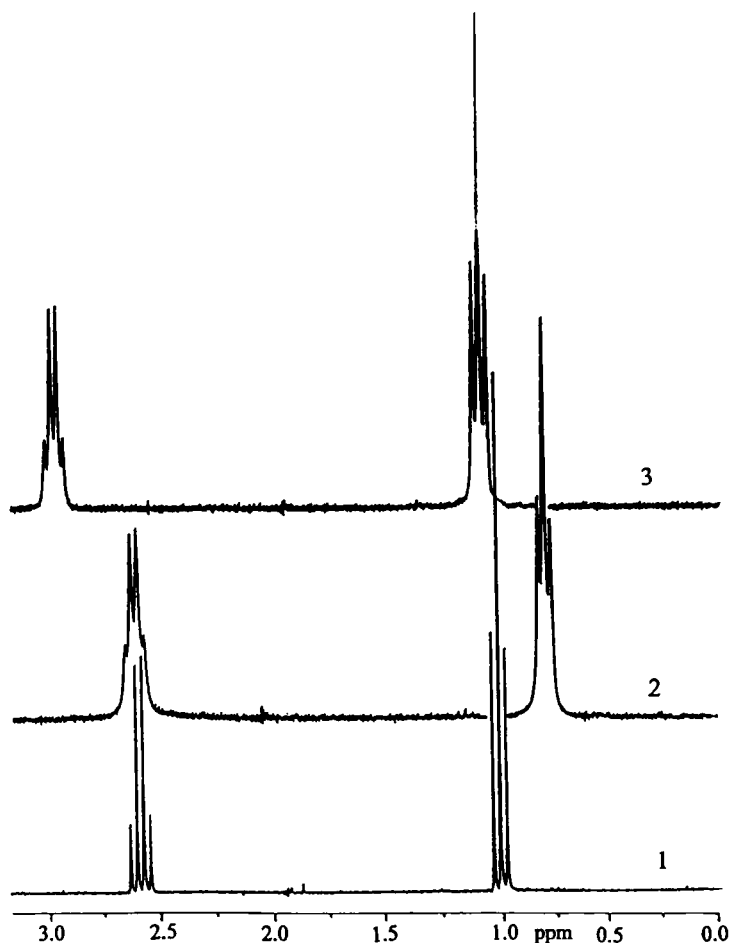
FIG.5. NMR spectra : 1 – \text{N}(\text{C}_2\text{H}_5)_3 amine, 2 – amine + 1, 3 – amine + 2.
